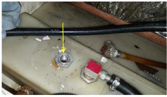
The fuel filling and vent lines were both marked ISO7840 and connected to the top of the tank. They led to a combined filling and vent fitting located on the starboard topside; all were in good condition.
