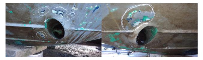
There were various area of exposed GRP on the lifting strakes, possibly due to chipping of the gelcoat when launching/recovering on the trailer. The areas are as follows:
