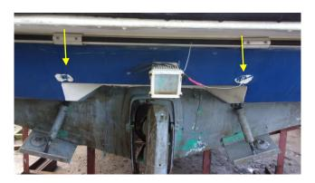
An LED lamp was fitted on the aft coaming to illuminate the bathing platform. This had come loose so should be secured.
